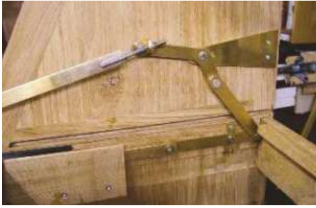
▲ Pic.11 The loper mechanism in its open position. Experiment with a mock-up made from offcuts until everything works correctly
